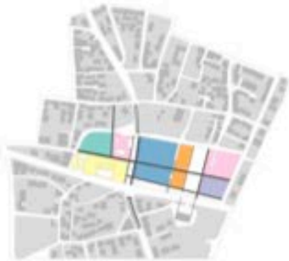
STEP 5: SETTING A CLEAR ZONING ACCORDING TO THE SURROUNDINGS AND THE NEEDS zoning pink residential 4000m2 + 7000m2 blue commercial + offices 4300m2 orange community center 5400m2 dark blue sports 13,700m2 yellow cultural 10,000m2 teal fresh market coop 5000m2
